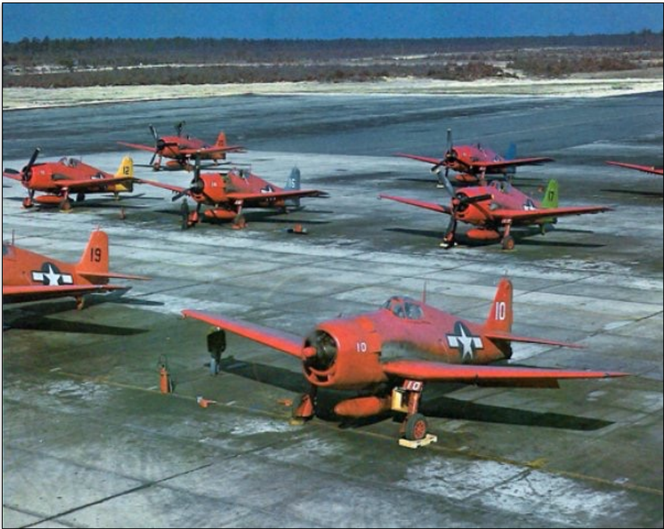
US Navy Grumman F6F-5K Hellcat drones , with their tails painted different colors to indicate different radio guidance frequencies, await the call on Roi Island during Operation Crossroads. (Library of Congress)
